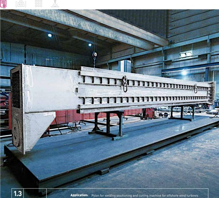
Made to measure WELDING Application:<br/>Steelgrade:Pylon for welding positioning and cutting machine for offshore wind turbinesSteelgrade:\$235JR / \$235JRG2Weight / Dimensions:<br/>Particularity:15,6 to / 1,550 x 2,150 x 12,286 mmFlatness and dimensional accuracy of the overall construction, welds inside the<br/>component (confined space) and mechanical processing
