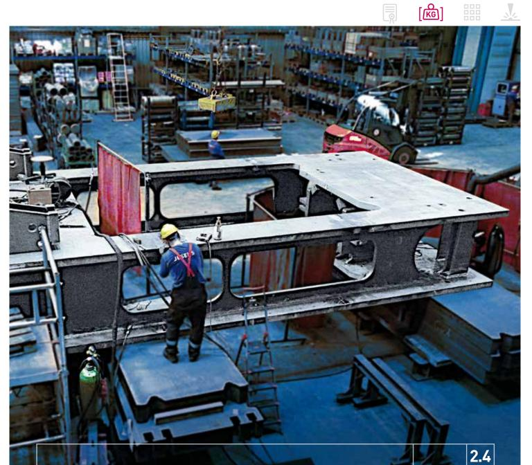
Application:Press frameSteelgrade:S235JR+NWeight / Dimensions:44.2 to / 2,600 x 3,910 x 7,858 mmParticularity:Frame sheet UP-welded, flatness frame sheet and mechanical finishing
