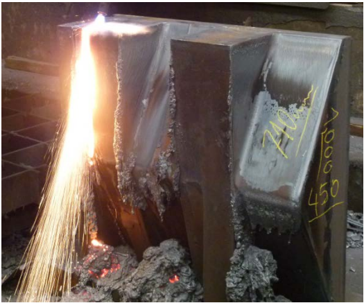
Picture 4: From a steel block 450 mm thick and 1,000 mm high, four diagonals separated by a bar – in parallel pairs – were cut.
