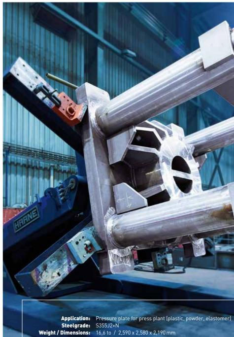
Particularity: Tolerances of the column guides and mechanical end processing
