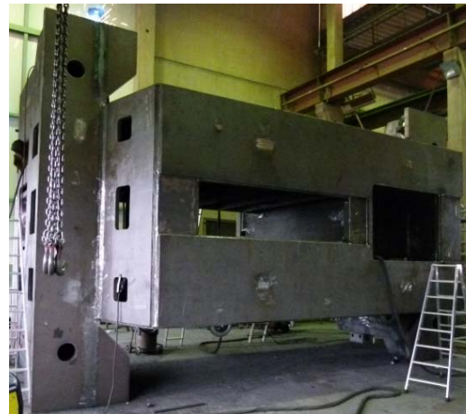
Image 4: Precision and Performance: The production of the press table was a real challenge for the welding experts from Korntal-Münchingen.
