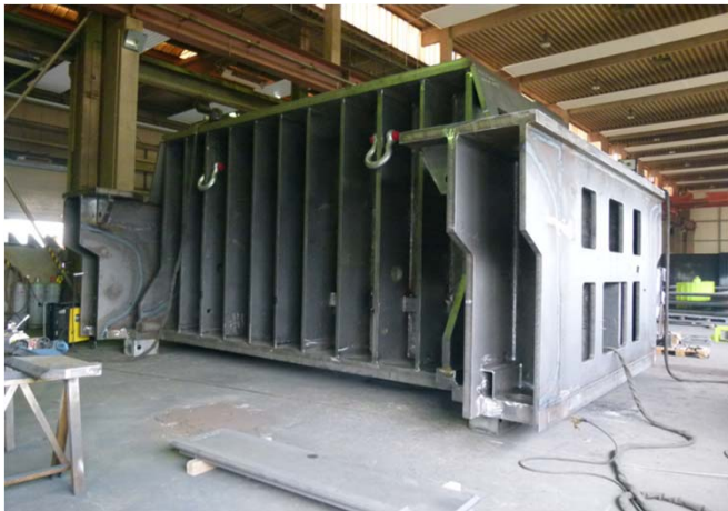
Image 3: Precision work in steel: While producing the 156-tonne colossus, the welding experts from Korntal-Münchingen had to adhere to minimum tolerances.
