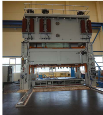
Image 6: Jebens manufactured the welded components for the more than 8 meters long press table exactly as per customer specifications.
