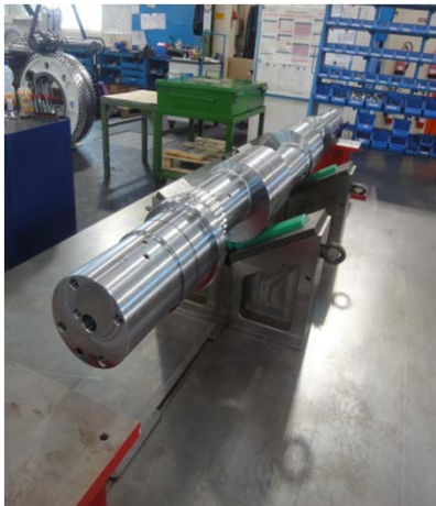
Images 12 - 13: Special stability: The power unit with the quadruple stored eccentric shaft plays a decisive role for stability, absence of vibrancy and lifetime of the Jebens press table.
