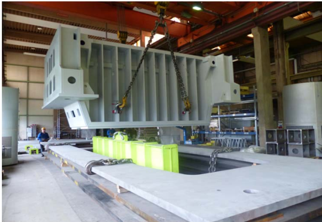
Image 5: Colossus in perfect grip: Handling the 156-tonnes components was a job of precision.
