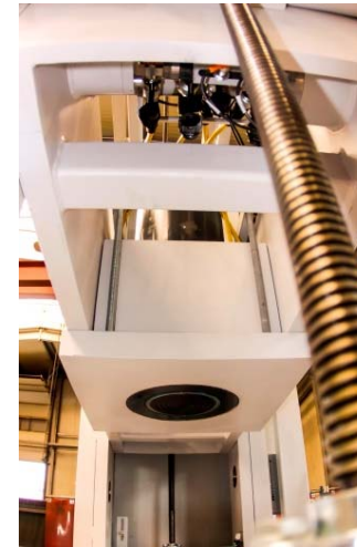
Picture 8: The hydraulic cylinder mounted centrally in the upper yoke locks automatically in the new position.
